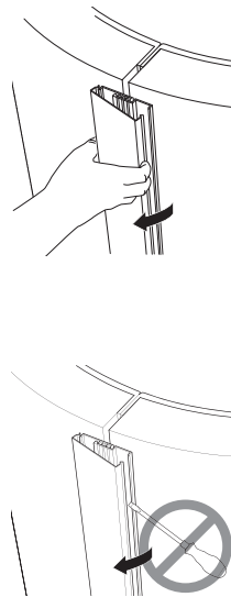
Do not use any tools when dismantling the joining plate.
